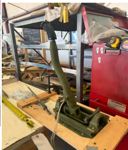
Left: John Flynn completed the fabrication of the mounting base/mechanism for the control stick.
