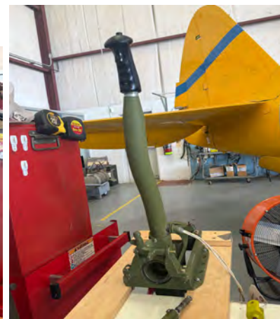
Left: John Flynn completed the fabrication of the mounting base/mechanism for the control stick.
