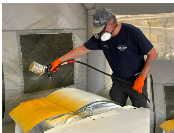
Col Roy Handler sprays the first coats of yellow on several Stearman parts.
