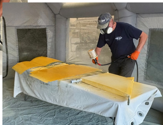
Col Roy Handler sprays the first coats of yellow on several Stearman parts.
