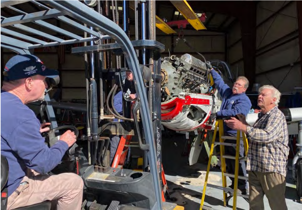
Cols Rodney Higginbotham, Dennis Beach, Tom Langford, and Bill Freyman remove the Merlin engine from Red Nose. The replacement has already been uncrated and will soon be installed. →
