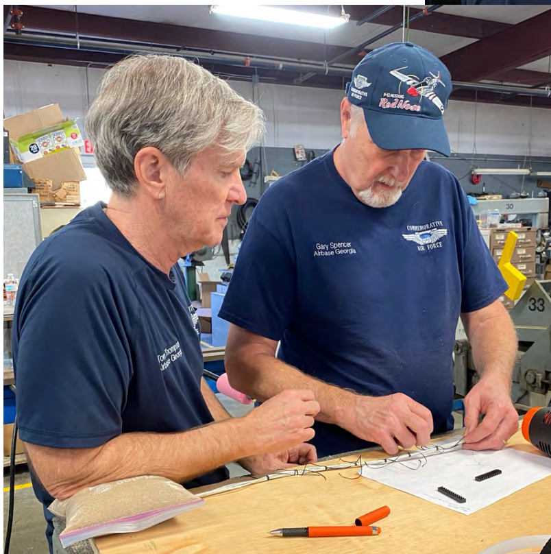
Left: Cols Tom Thompson & Gary Spencer assemble a wiring harness for the P-47.
