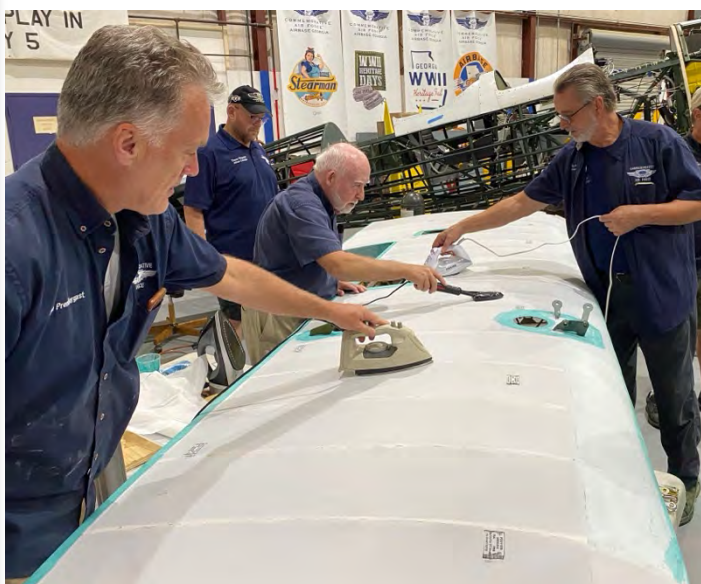
Cols Jim Prendergast, Malcolm Lelliott, Thomas Pfingsren & Roy Handler work on shrinking wing fabric.
