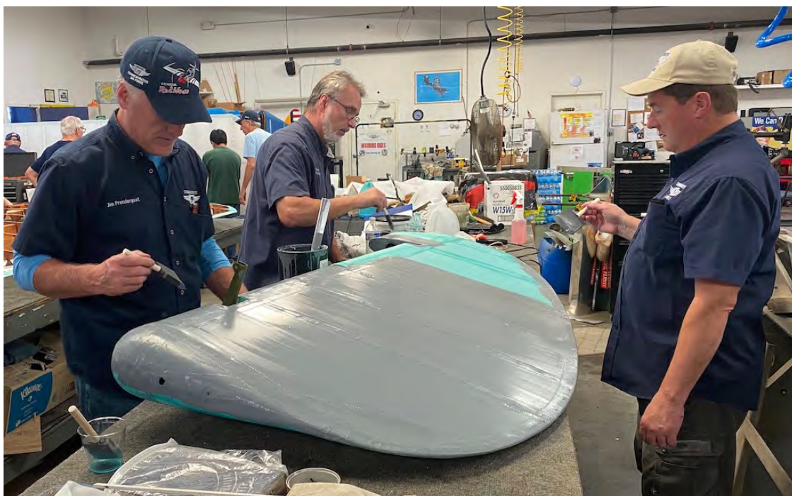
Below, L-R: Cols Jim Prendergast, Roy Handler & Chris Buzzeo applying first coat of primer.
