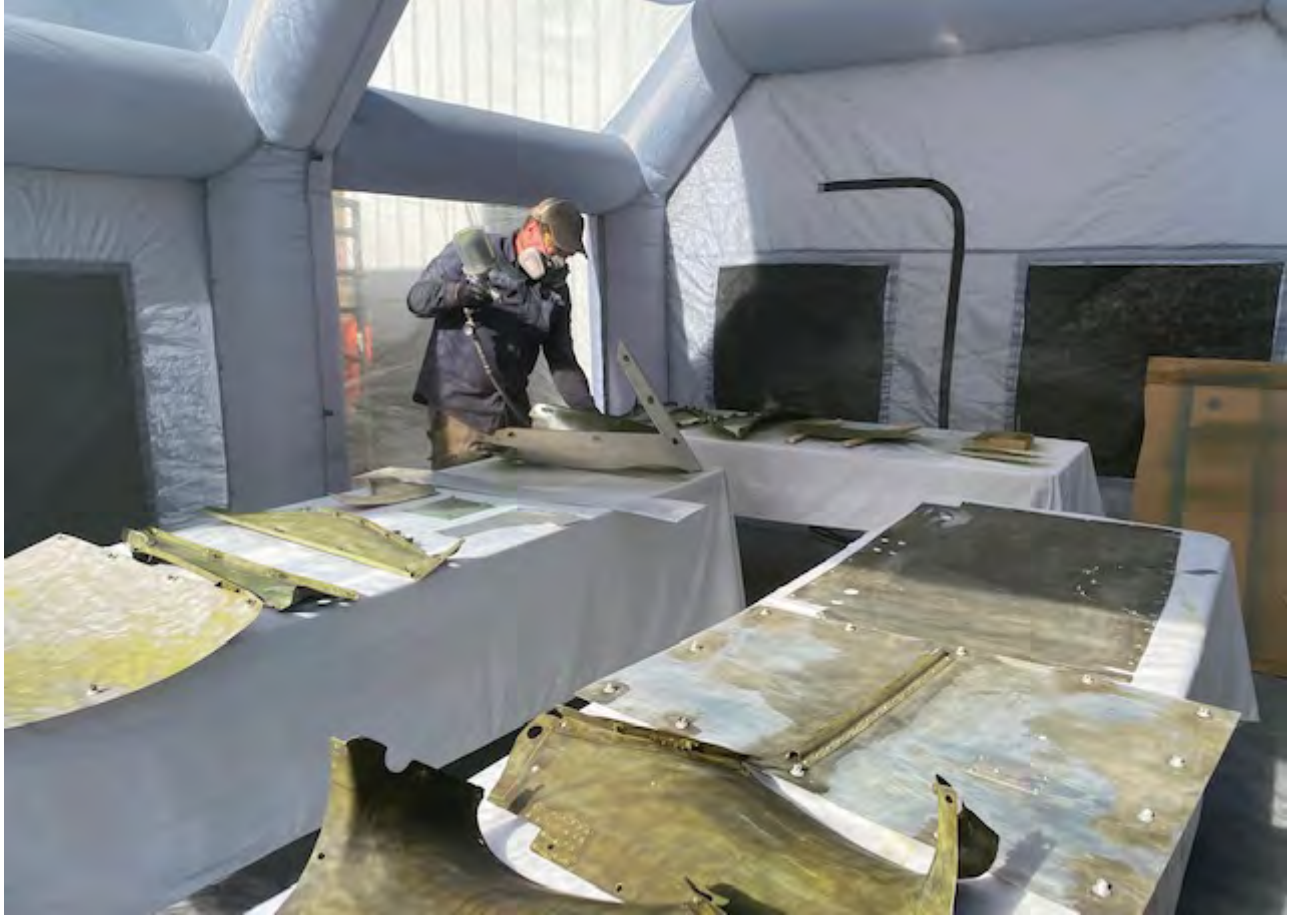
Above: Col Chris Buzzeo sprays 1st coat of primer on Stearman parts.
