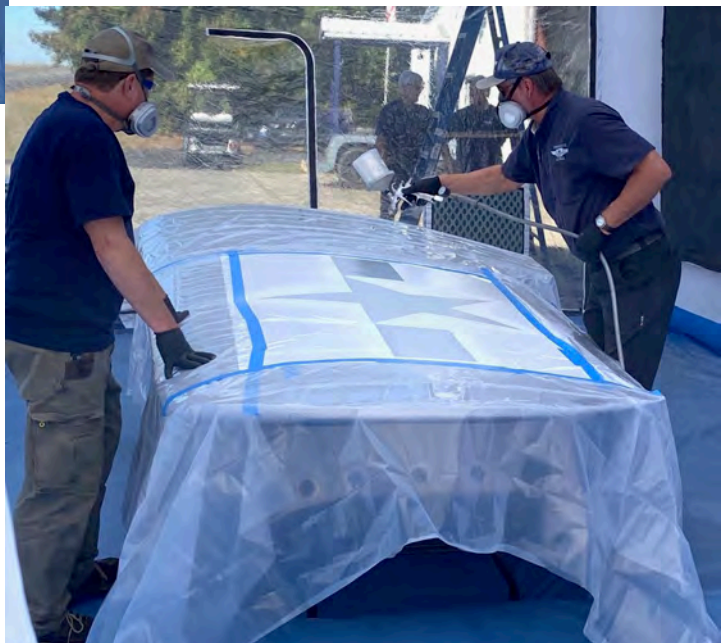
Right: Cols Chris Buzzeo & Roy Handler paint the white portion of the National Insignia on the wing.
