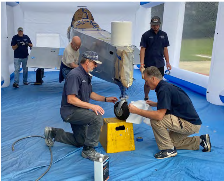
Cols Roy Handler & Jim Prendergast (kneeling) mask off the tail wheel while Cols Gary Spencer, Forest Buchanan & Cadet Arthur Richez do a wipe down before final silver color coat is applied.
