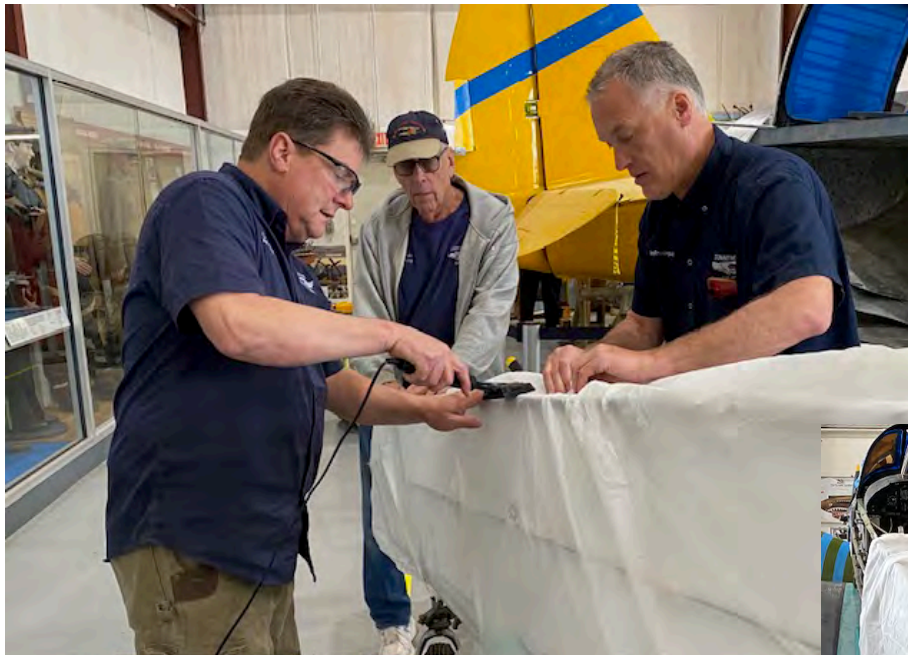
Cols Chris Buzzeo, Paul Brunks, and Jim Pendergast work on covering the fuselage with fabric.
