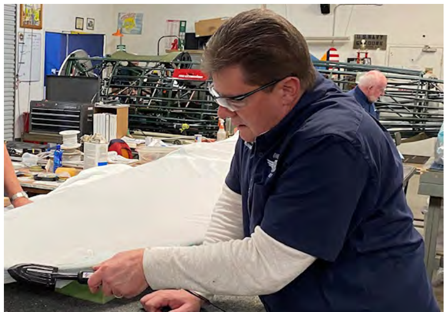
New Col Gary Spencer helps Col Roy Handler smooth out new fabric on horizontal stabilizer, preparing to shrink & glue fabric in place.
