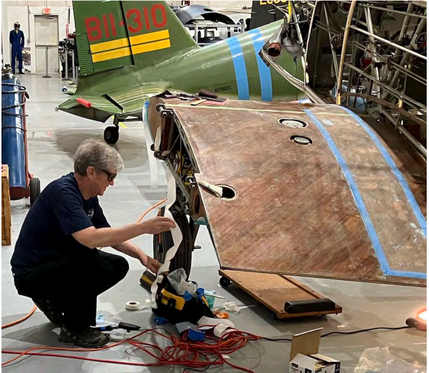
PT-19 Project Manager Col Tom Thompson works on preparing the left wing for fabric covering.
