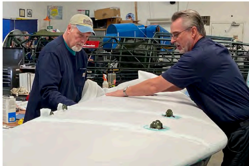
New Col Gary Spencer helps Col Roy Handler smooth out new fabric on horizontal stabilizer, preparing to shrink & glue fabric in place.
