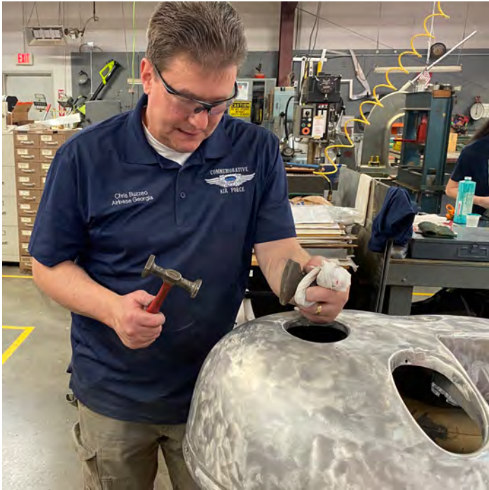
Col Chris Buzzeo Repairing & straightening nose cowl using body dolly & hammer.
