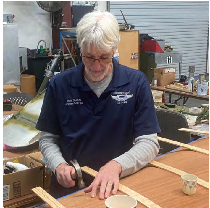
Col Mark Chabot temporarily tacks wooden strips in place to hold the shape of the horizontal stabilizer until the glue cures.
