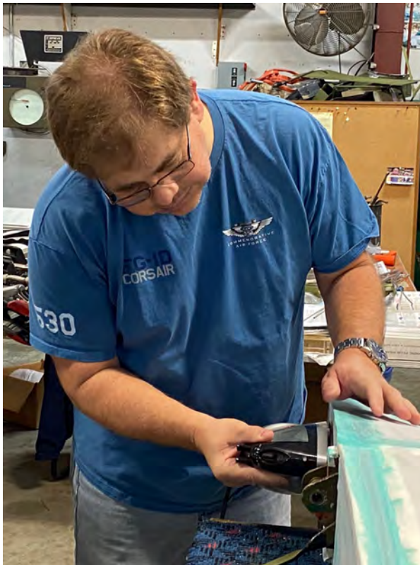
Col Mike Lamble irons fabric to make it taunt on center wing section
