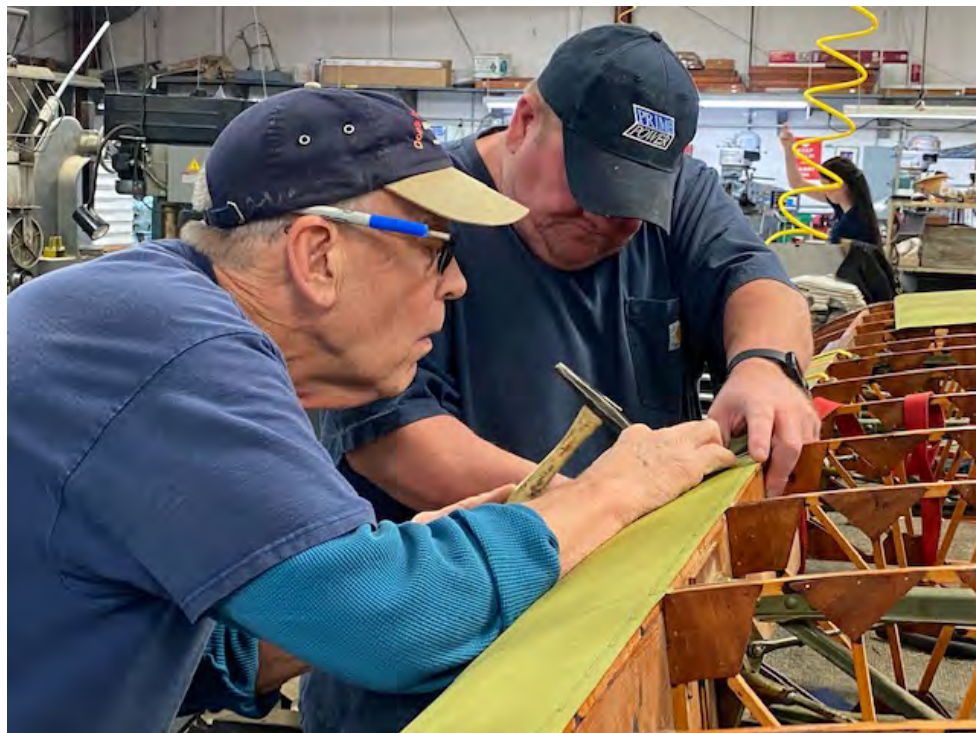
Paul Brunks & Wayne Cantrell attach (i.e. nail) leading edge metal to Stearman wing.
