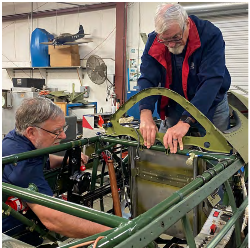
Although it doesn't look like it, Cols "Tagg" Taggart & Joe Broker are fitting the front cockpit seat in the Stearman .
