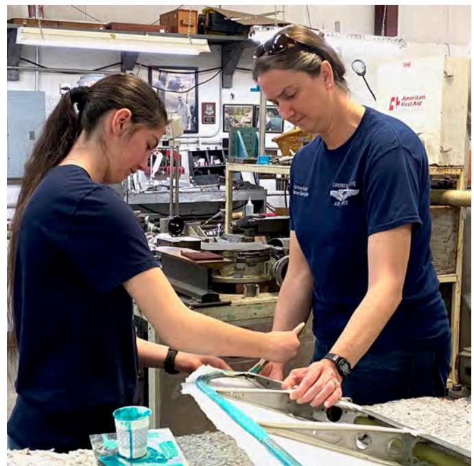
Yvonne Haley & daughter Ann work on covering the elevator.
