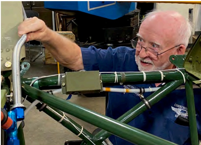
Left: Col Malcolm Lelliott test fits the fuel line that will run from the upper wing down to the selector valve.
