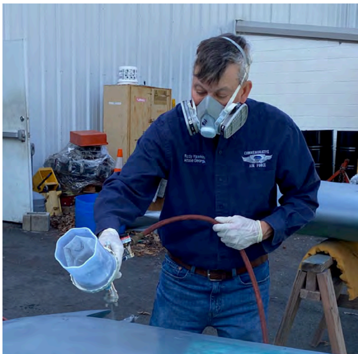
Left and below: A PT-19 wing gets a primer coating from Col Randy Hawkins.
