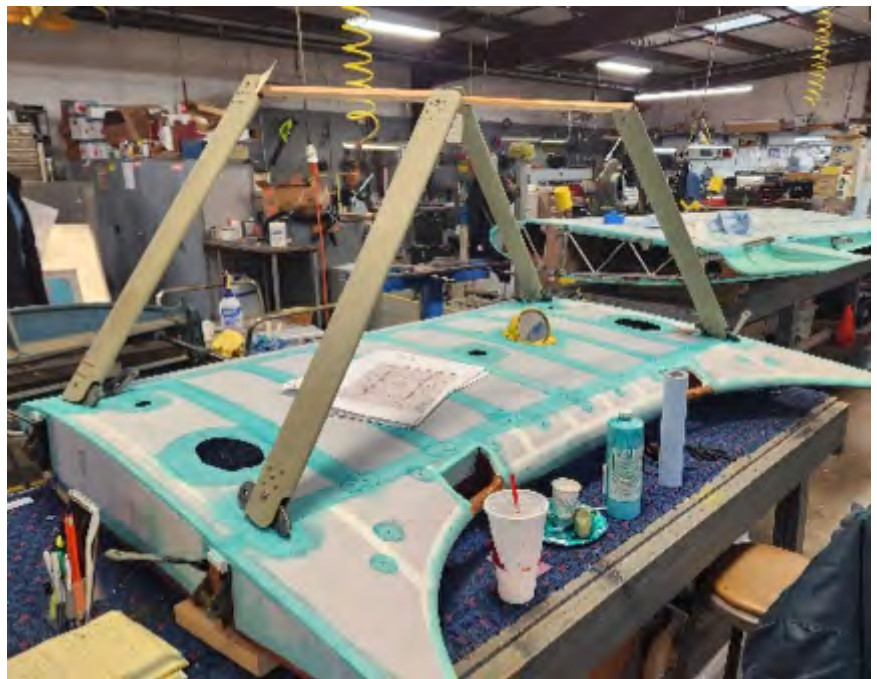
Bottom covering complete (with cabane struts temporarily installed for fitting).
