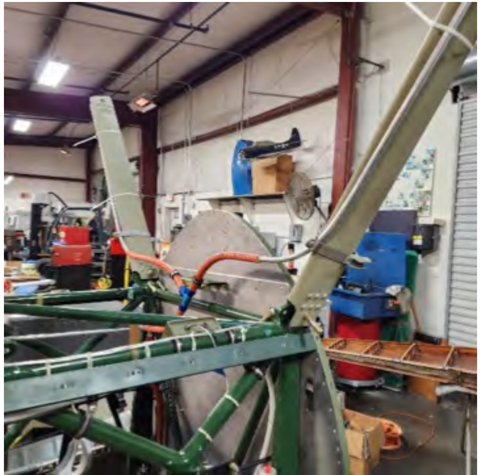
Left: Col Malcolm Lelliott test fits the fuel line that will run from the upper wing down to the selector valve.
