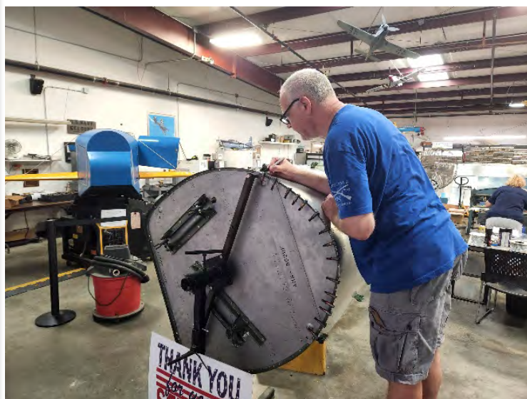
Above: Col Brad Postage fabricating sheet metal for the fuselage. The new firewall is also visible.
