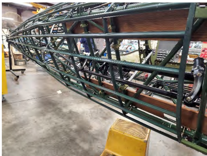
Left: Lower Birdcage – repaired and installed.
