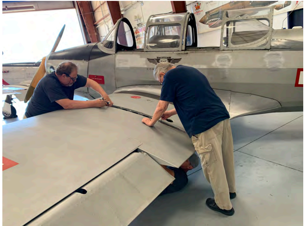
Above: Cols Steve Beck and Lee Walker remove the wing attachment bolts from the aircraft.
