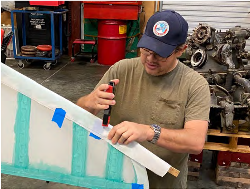
Col Mike Lamble works on the Stearman's fabric covering.
